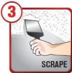
Use a scraper blade to remove softened texture, taking care not to damage underlying surface. Catch the removed softened texture in a painter's tray and discard safely.
